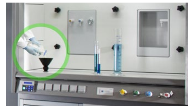
Figure 5 Schematic diagram of a funnel with a discharge pipe and level monitoring for installation in a fume cupboard. With a comprehensive approach at the planning stage, the proper handling of hazardous substances, as well as their storage and disposal, will be made easier for the later users of the laboratory.
