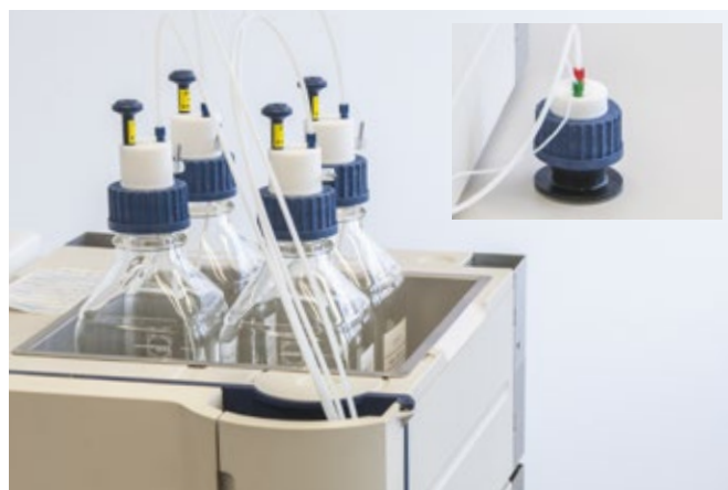
Figure 2 Arrangement for HPLC waste collection with collector fitting, collection container and level monitoring
