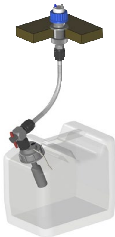
Figure 2 Arrangement for HPLC waste collection with collector fitting, collection container and level monitoring
