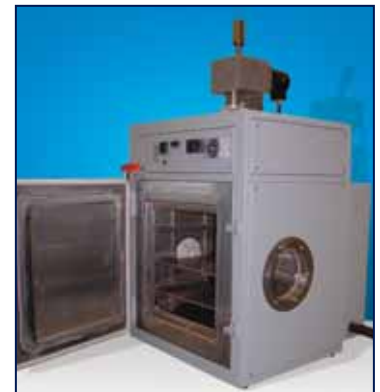
THREE CUSTOM MADE CYLINDER WARMING OVENS EACH DESIGNED TO OPERATE IN A ZONE 2 HAZARDOUS AREA & CERTIFIED TO EU ATEX DIRECTIVE 94/9/EC. EACH CHAMBER ACCEPTS FIVE 1620x255mm CYLINDERS
