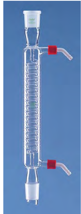
Spiral-condenser with GL Thread
