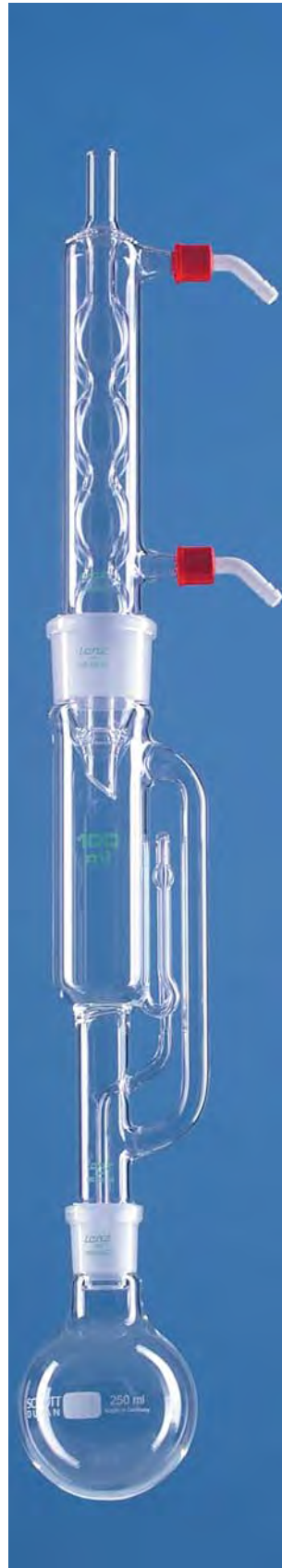
Soxhlet Extractor with Allihn Condenser
